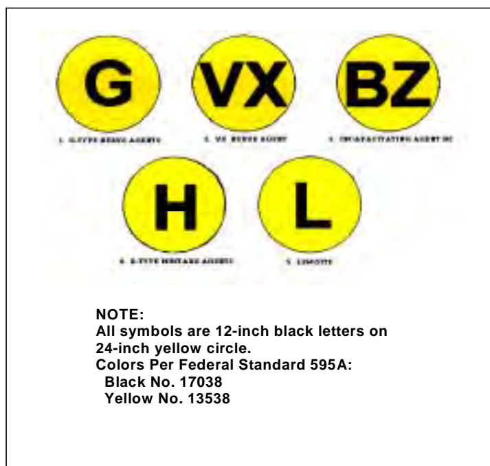
Figure 8-5. Supplemental Chemical Hazard Symbols
